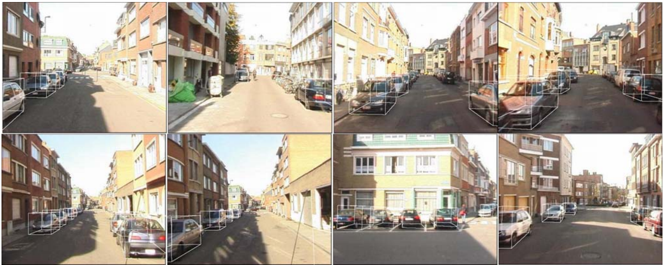
Fig. 16 (top) Online 3D car location estimates of our system using only information from previous frames. (bottom) Final 3D estimates integrated over the full sequence
