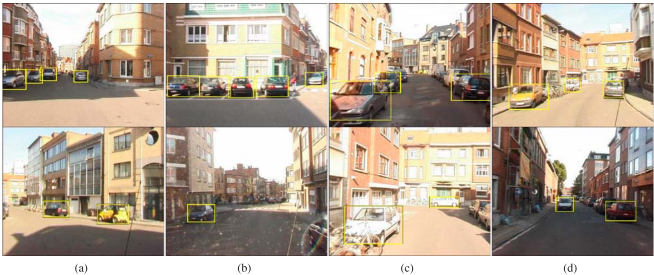
Fig. 14 (top) Car detections on typical images from the city scenario. (bottom) Examples for the difficulties in this scenario: a motion blur, b lens flaring, c bright lighting, d strong shadows
