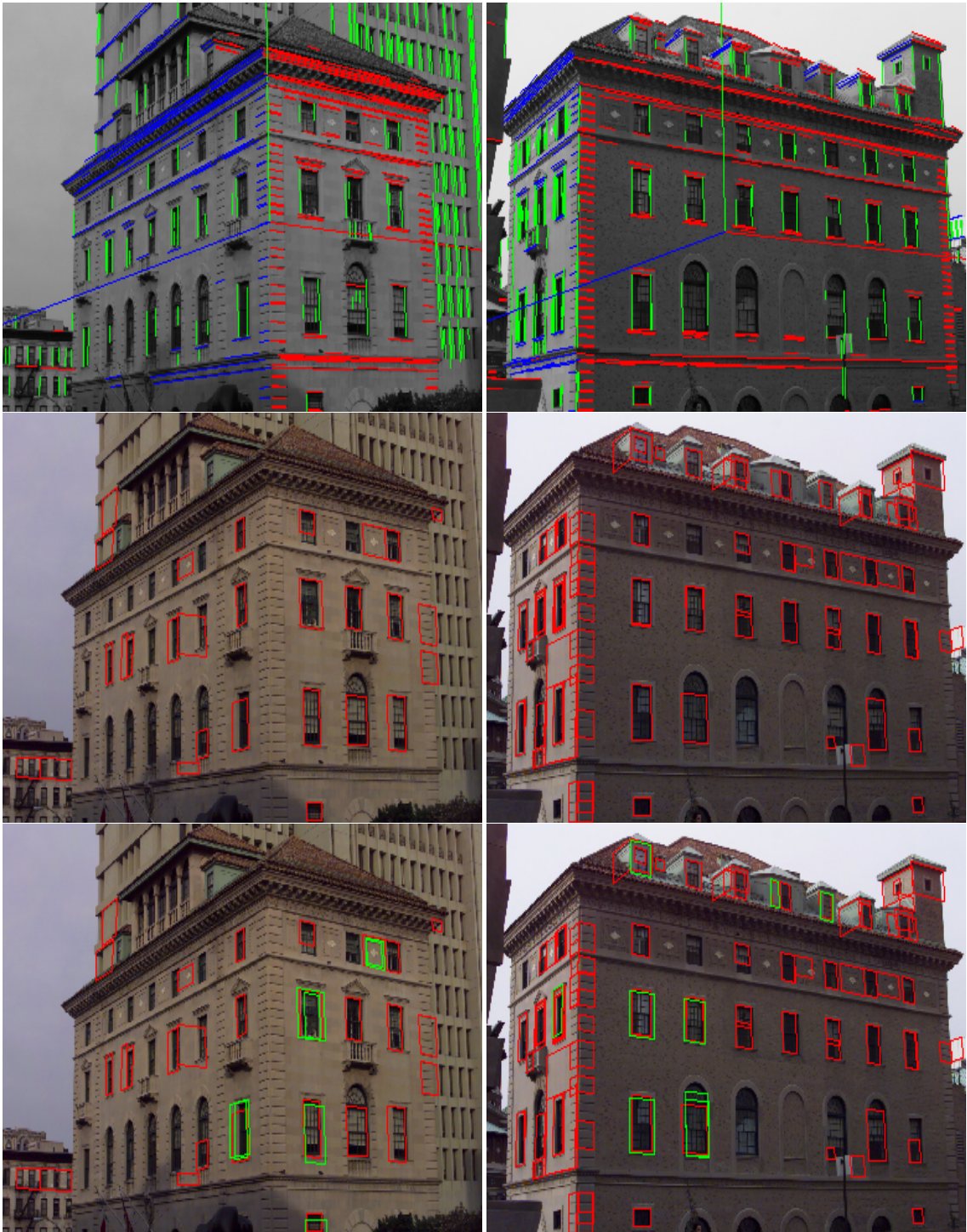
Figure 5.15: Results. a,b) 2-D images and clusters of 2-D lines, where different colors correspond to different vanishing points. c,d) Extracted 2-D quadrangles (two views). e,f) Extracted 2-D quadrangles (shown in red) and Q_{match} matched 3-D rectangles projected on images after coarse pose estimation (shown in green).
