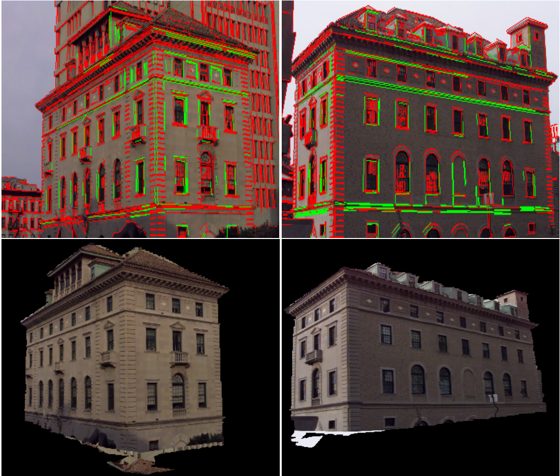
Figure 5.16: Results. a,b) Projected 3-D lines on the images after final pose estimation (shown in green). The extracted 2-D lines are shown in red. c,d) Images texture-mapped on 3-D model assuming final pose.
